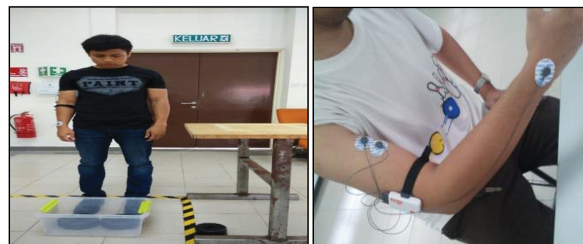
Figure 5. Shimmer EMG electrode placement and lifting setup
